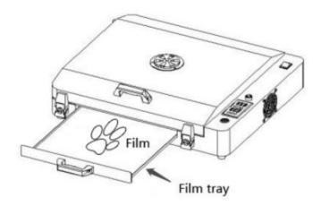
3.1 Put the picture film into the tray for baking and colour fixation. After curing, take out the curing tray, take out the film in the tray, and curing is completed.
